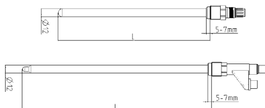
Fig. 9 Sensor filled with gel (top), sensor filled with liquid (bottom)
